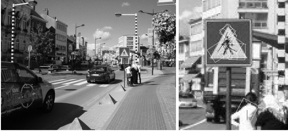
Figure 7: Typical experimental results. In a query image, all matching visual words are shown for the pedestrian crossing sign (white squares). From each visual word, the anchor location is computed (black line pointing from visual word centre to anchor). The zoom on the right shows clearly the recognised sign: many anchor lines coincide.
