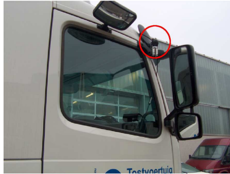
Figure 6: Our blind spot camera mounted on the test truck.
