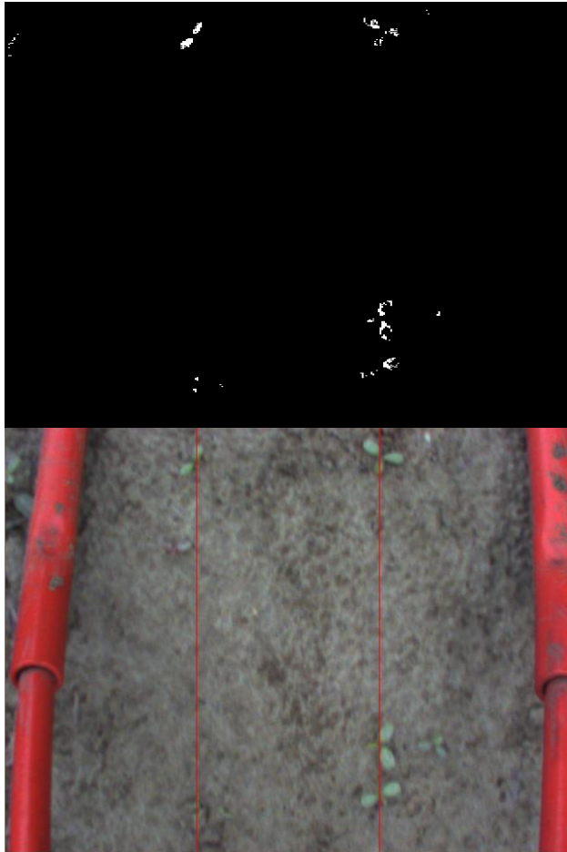
Figure 14: Illustration of the Belgian chicory results. Above: segmentation results of one camera image. Below: original camera image with superimposed the two estimated crop row positions (red).
