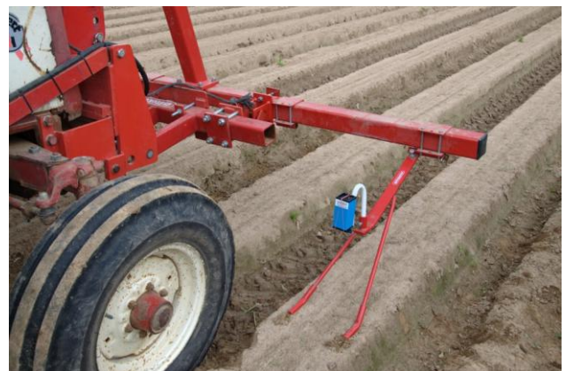
Figure 13: Test field for Belgian chicory, showing our camera mounted on an agricultural machine
