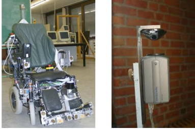
Figure 1: Left: the robotic wheel chair platform. Right: the omnidirectional camera, composed by a color camera and an hyperbolic mirror.
