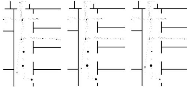
Figure 13: Three belief update cycles in a typical localisation experiment. The black x denotes the location of the new image. Place prototypes with a higher belief value are visualised as larger black circles.
