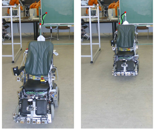
Fig. 6. Target position (left) and start position (right) of the wheel chair, with superimposed projected motion (black: without structure, light green: using structure).
